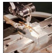
Wire Bonding a Quantum Cascade Laser on a C-Mount
